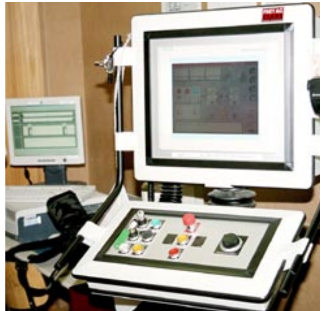
Operational Controls (right) and Visualisation (left) are separated intentionally to keep the operations monitor as clear and simple as possible
