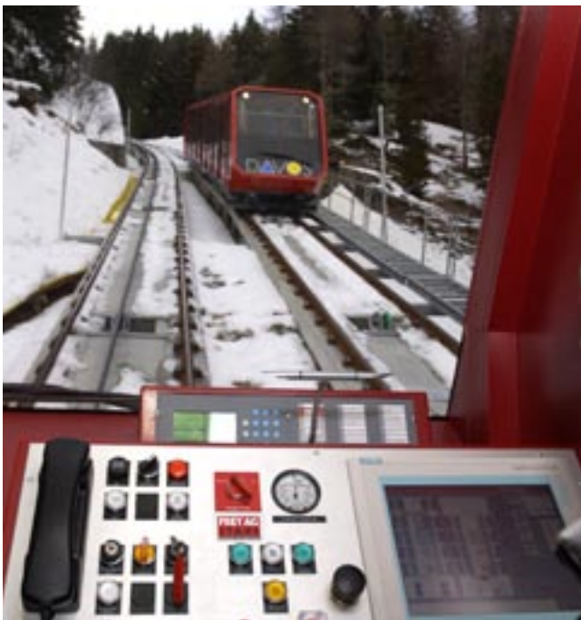
200 passengers are transported from 1557 m up to 2218m a.s.l. in 253 s. Nominal power of 1250kW is required for that.
