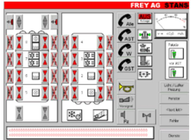
Monitor display in the cars. The operator sees all important information including a first fault text display
