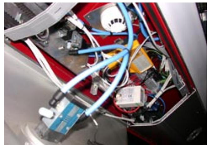
Remote I/O modules (yellow) in the roof compartments for door and compartment controls.
