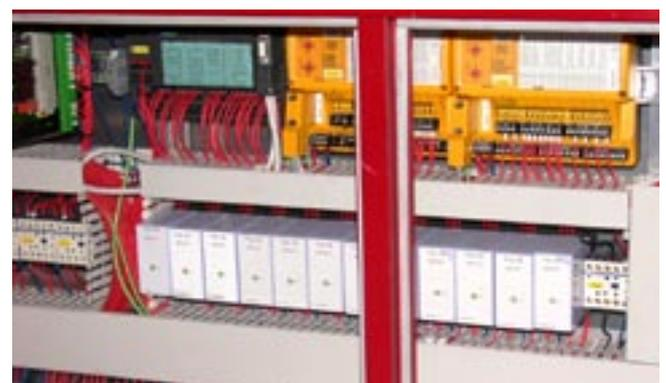
Control cabinet in upper drivers compartment with PSS I/O modules, S7 Profibus controller and common vehicle electric. Layout is clear and maintenance friendly.
