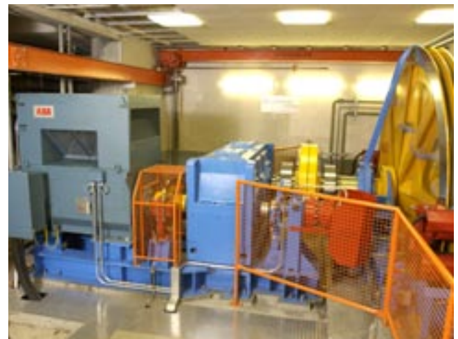
AC drive squirrel cage motor with gear box..
