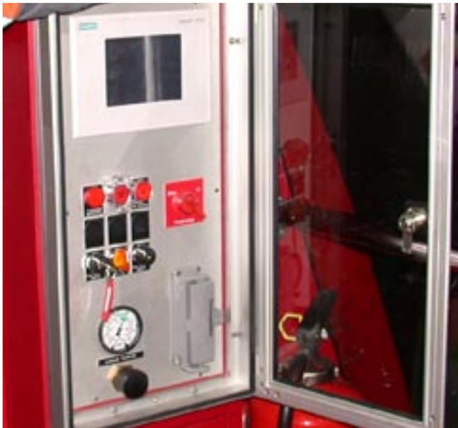
Downhill side emergency control station with touch panel and important controls and indications. This control station is normally locked..
