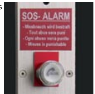
An Alarm button is mounted in each compartment. Activation will alert the driver.
