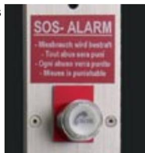
An Alarm button is mounted in each compartment. Activation will alert the driver.
